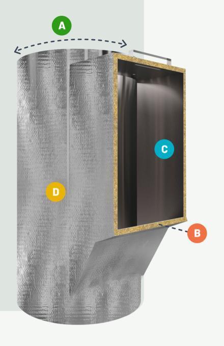
A minimum 2mm Sound deadening coating applied on the exterior of the chute in order to inhibit any unwanted noise from falling garbage inside the chute. Optionally, an extra 25mm foil faced fiberglass insulation coating is wrapped around the exterior of the chute.
